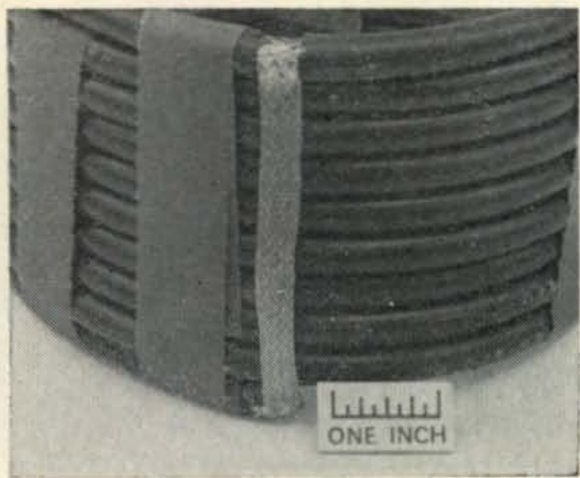
Fig. 6—The outer conductor of the balun coil is jumpered to itself at each end of the coil. This is a common ground point and may be connected to the metal boom of the beam antenna. A short length of copper braid was used in this balun, but a length of copper strap may also be used.
